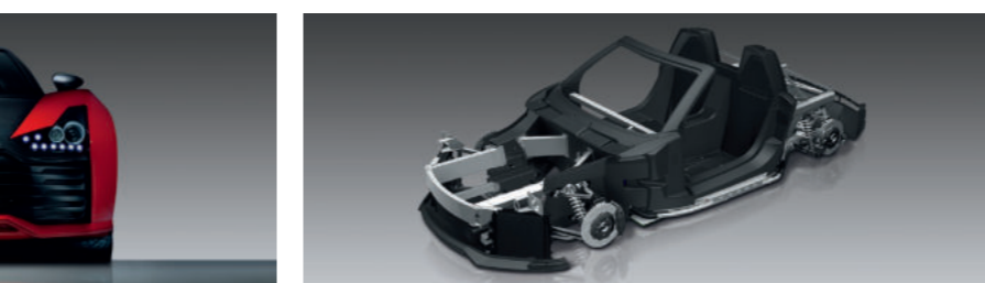
From: Roding Automobile GmbH Roding CPK-chassis made of AH 140 from vacuum infusion
