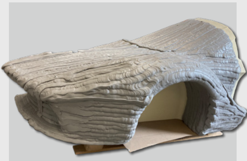
Full scale automotive design model produced with P29. Paste applied by ebalta team.
